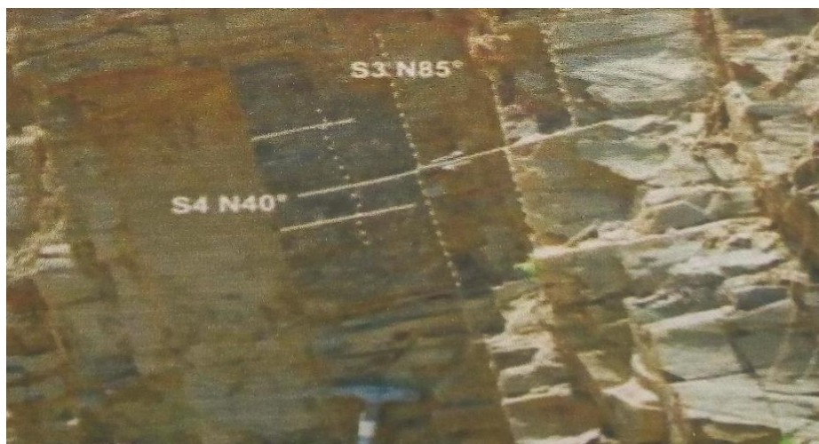
Figure7. Schistosity of S3 fracture, sub-vertical, oriented from N800 to N100 removed towards the right side by another S4 schistosity slightly leaned, with a N400 direction.
