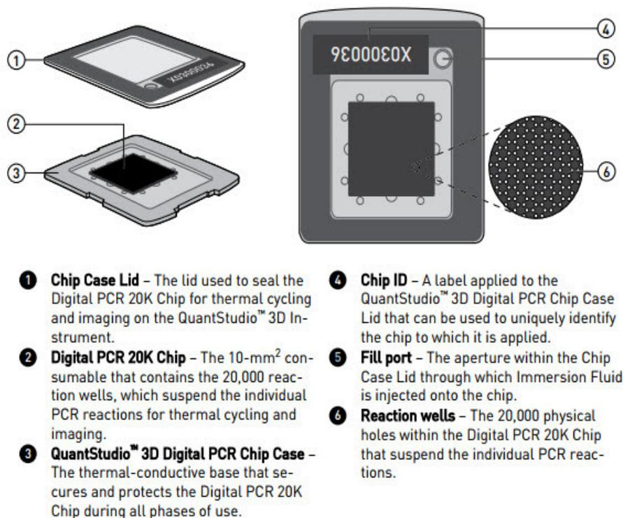
**Figure 2.** Diagram illustrating QuantStudio™ 3D Digital PCR System Chip; ChipCase Lid (1); Digital PCR 20K 10 mm<sup>2</sup> nanofluidic v2 chip (2), which contains 20,000 reaction wells; QuantStudio™ 3D Digital PCR Chip Case (3); Chip ID (4); Fill port (5); and Reaction wells, the 20,000 physical holes that suspend individual PCR reactions (50).
