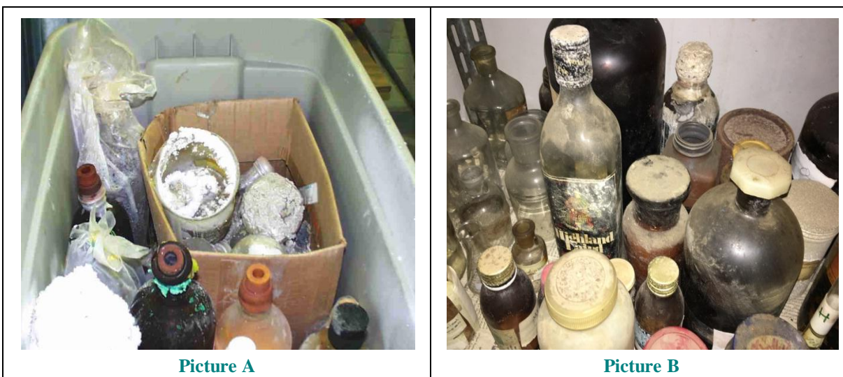
Figure2 (Picture A, and B). Use of non-suitable bottles to conserve chemicals
