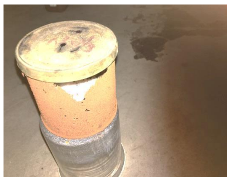
Figure4. Sodium azide found in a metal box and has been corroded
