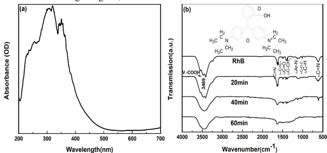
**Fig3.** UV-Vis (a) spectra of  $\text{Cu}_3\text{Mo}_2\text{O}_9$  and FTIR(b) spectra of the degradation products of RhB at the different times.
