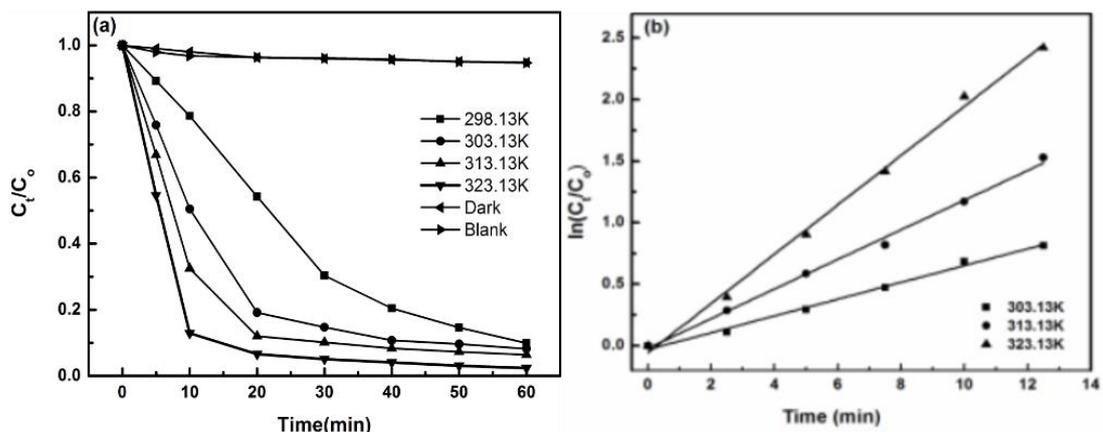
**Fig4.** Photo catalytic decolorization kinetics of RhB using Cu<sub>3</sub>Mo<sub>2</sub>O<sub>9</sub> as photocatalyst. The change in reactant concentration versus irradiation time is show as (a) linear and (b) logarithmic plots.
