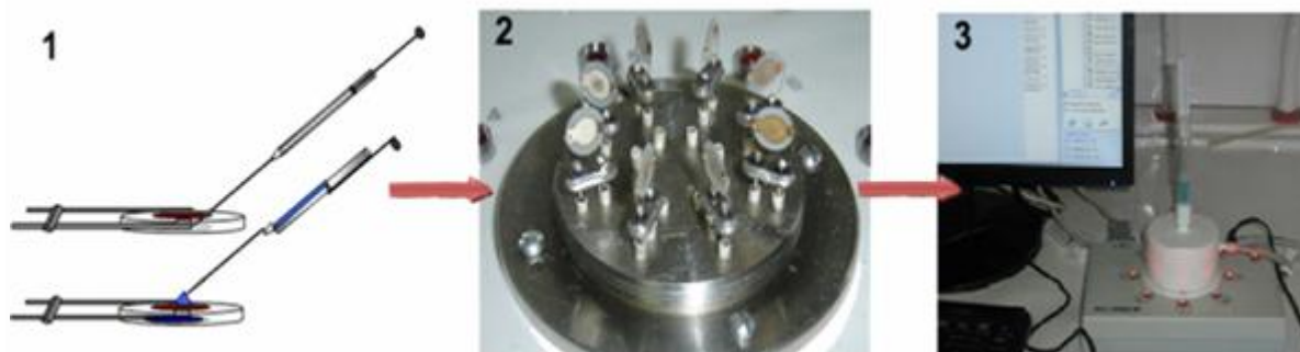
Fig1. Preparation of detection device: 1 – modification of piezoelectric quartz resonators electrodes; 2 – forming of sensors array; 3 – airtight detection chamber
