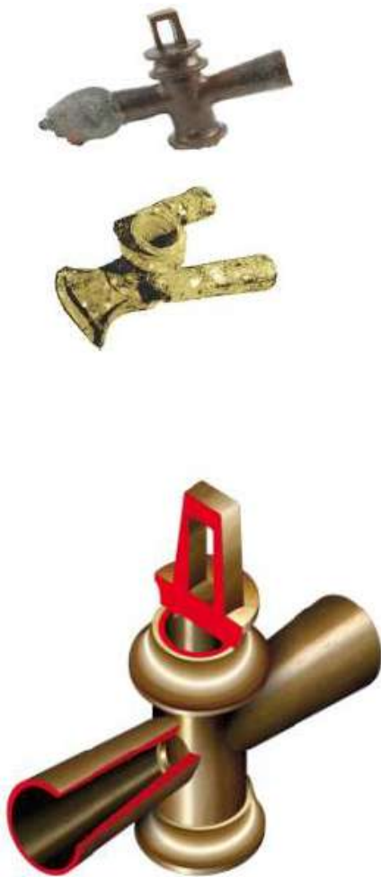
Figure15. Bronze arrest valves found in Herculaneum and still functional. Drawing illustrating of the valve
