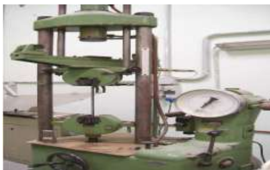
Figure10. The LOSENHAUSENWERK UPH10 testing machine used for experimental tests
