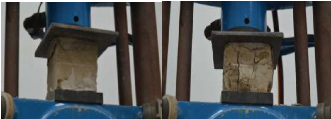
Figure 17. Execution of the compression test and failure of the specimen
