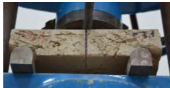
Figure12. Placement of the specimen into the testing machine
