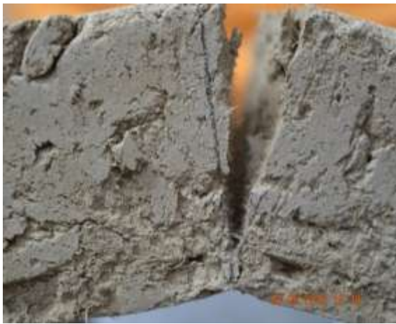
Figure 13. Bending failure of a tested specimen
