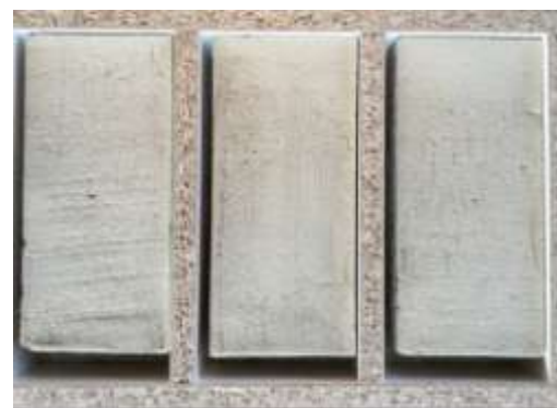
Figure9. Shrinkage effect of specimens in the timber formworks
