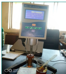
Figure 4. Viscometer, to measure viscosity at ambient and elevated temperatures.
