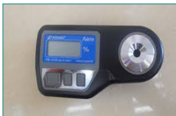
Figure 5. Refractometer, for measuring moisture content and total soluble solids.
