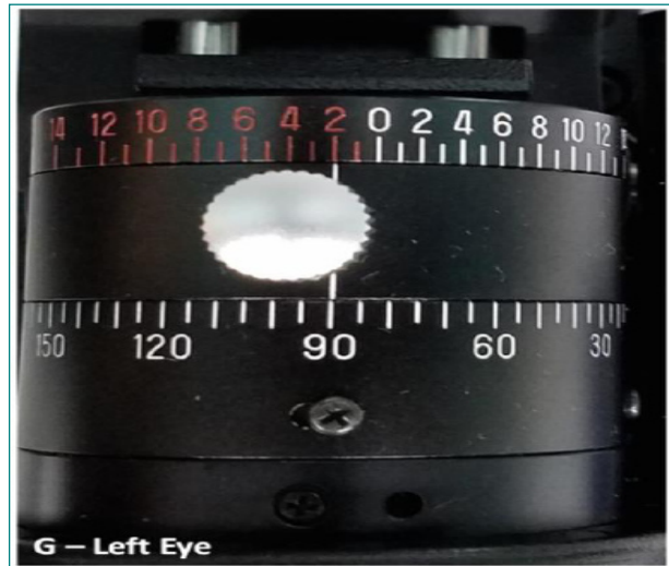
Figure 4(A-G). Measuring horizontal and vertical prism together
