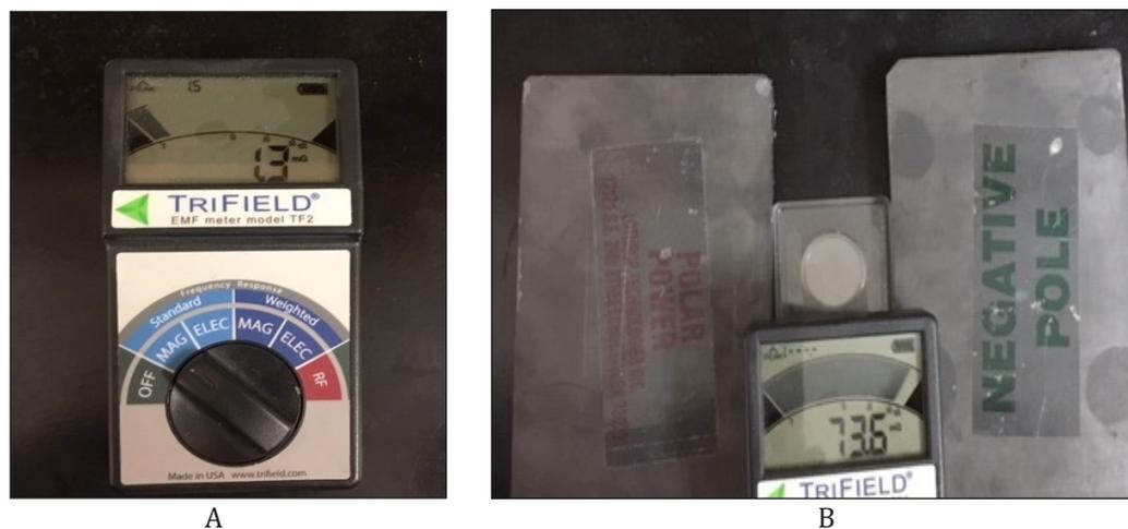
**Fig3. A.** Illustration of the TriField magnetometer. **B.** Two plate magnets placed on either side of the deep well slide containing the dwarf Stentor cells. See text for discussion.
