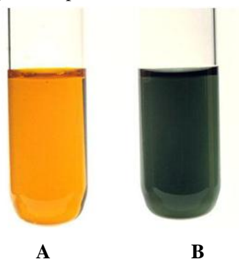
Fig3.3. Test for ethanol using acidified potassium dichromate solution (A) Colour for acidified Potassium dichromate solution (B) Colour for ethanol and acidified potassium dichromate solution after shaking.
