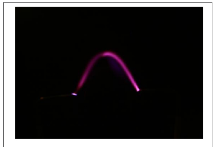
Figure 10. The form of a glow discharge at a pressure of 0.1 atm.
