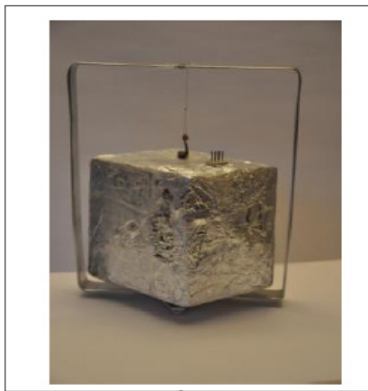
Figure 4. Fixed rotor of a mechanical aviation gyroscope with a horizontal axis of rotation
