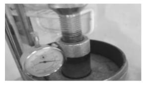
Figure6. Insert samples under the CBR device
