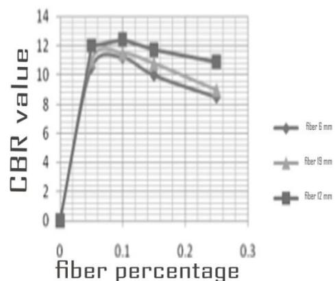
**Figure8.** Changes in the amount of CBR with different fiber percentages
