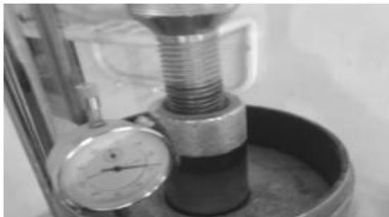
**Figure6.** Insert samples under the CBR device
