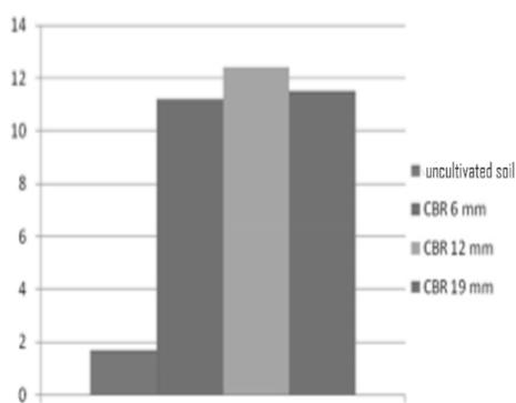
Figure9. Compare CBR value in different sizes of fibers
