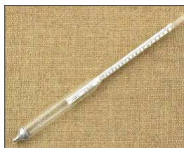
Figure 1. Hydrometer, for measuring the density of honey samples
