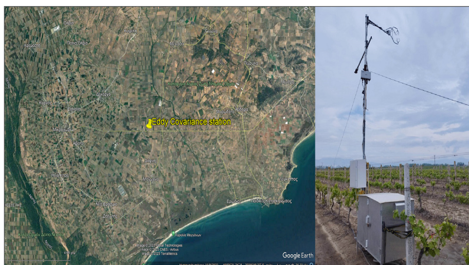
Figure 1. Micrometeorological eddy-covariance station at the Mangana “Merlot” vineyard (Eastern Macedonia and Thrace, Greece; Mercator zone 35 T; 320634 E and 4537472 N). Also, the CNR4 and logging and ground-based instrumentation are shown.
